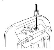
4. Route the modular cord through the wide right groove on the bottom of the bracket.
